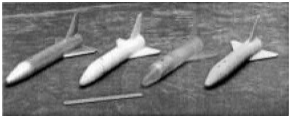
Fig. 2 Models tested (from left): aluminum, FDM-ABS, SLA, and SLS.
